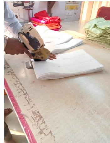
Plate 4.68: Cutting of fuse paper with electric rotary fabric cutter machine
